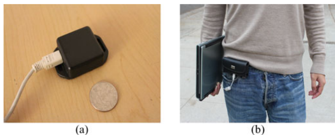
Fig. 1. MotionNode sensor and its placement. (a) MotionNode platform. (b) During data collection, a single MotionNode is packed firmly into a mobile phone pouch and attached to the participant's front right hip.
