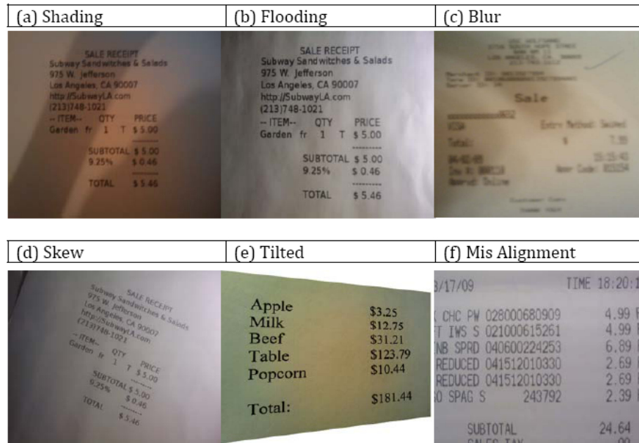
Fig. 1: Different issues arising in camera-captured documents: (a) shading (b) flooding (c) blur (d) skew (e) tilted (f) misalignment
