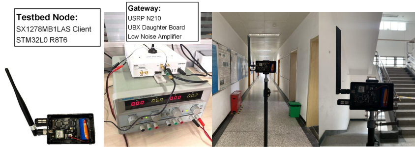
Figure 4: USRP N210 based gateway and commodity SX1278 client radio based LoRa node.
