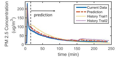
**Figure 7:** The illustration of the IAQ forecast algorithm in the context of predicting the PM 2.5 sensor values of a trial of pesticide spray.
