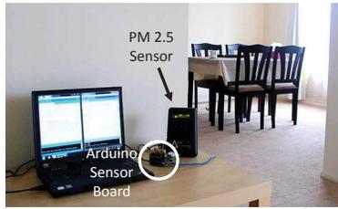
**Figure 13:** The deployment of AirSense in the living room at one home.
