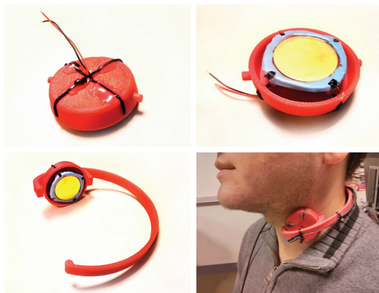
FIGURE 2. The top view (top left) and bottom view (top right) of the microphone with suspension capsule. It also shows the neckpiece design (bottom left) and how it fits on a person's neck (bottom right).
